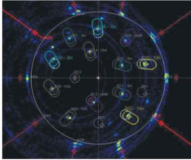
RAMS™ can be used as a supplement to many of these proven technologies and in some cases may be used as an alternative. Unlike many of these technologies, RAMS™ provides real-time imagery and status monitoring of the integrity of the mooring lines, umbilicals and risers, generating an alarm if the system identifies abnormal movement of the target. It also provides trending data that can be used for long term analysis. RAMS™ does not require sensors mounted to individual targets.
