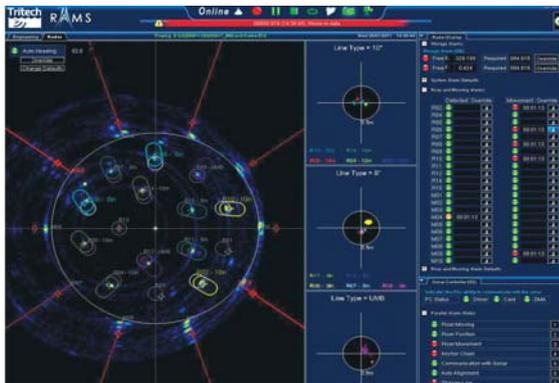
Image showing RAMS™ software screen; here a simulation shows potential alarms in Riser Movement, Anchor Chain, Storage Low and Noise.
